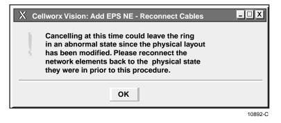
Figure 738-8. Add EPS NE - Reconnect Cables Instructional Window
